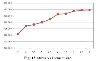
The optimum mesh size is determined by analyzing case 1 to 10 with Centre hole diameter = 100 mm and adjacent holes diameter = 50 mm. The maximum stress converges between mesh size 2.5 and 2. Hence mesh element size 2.5 will be used for the further analysis.
